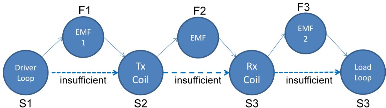
The above Su-Field model is the model that the team finally used in the solution generation for this issue. Now that we have a good Su-Field model we have to identify the SIS to be used in the solution concept generation process. If you have had Level 2 TRIZ training you may recall that there are five classes of SIS: 1.)birth/death, 2.)growth, 3.)marriage 4.)measurement and detection and 5.)how to
